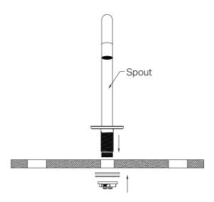
4. Insert the spout into the counter-top hole. Reattach the rubber washer, metal washer, and locking nut underneath the counter-top.
