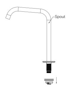
2. Remove the locking nut, metal washer, and rubber washer from the spout.
