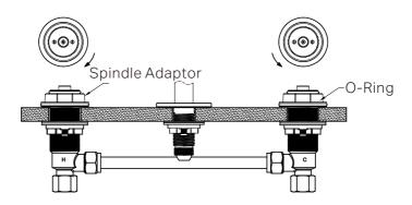
8. Apply lubrication evenly to the O-Ring. Refer to the diagram to identify the correct O-Ring position. Ensure the O-Ring is well-lubricated to prevent damage during installation.
