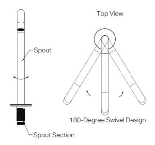
3. Secure the spout assembly at the spout connection. Rotate the spout to the desired position and align the spout approximately to the center of its rotation range.
