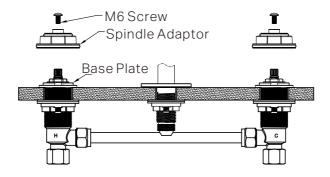
7. Screw the spindle adaptors onto the spindles and secure them with the M6 screws.
