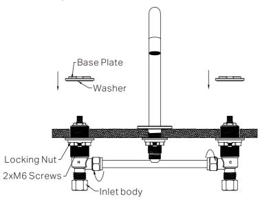
6. Insert the body set from underside of the counter-top. Using base plate and M6 screws to securing the body set, ensuring a firm connection. Ensure the washer is properly seated between the base plate and the body set.
