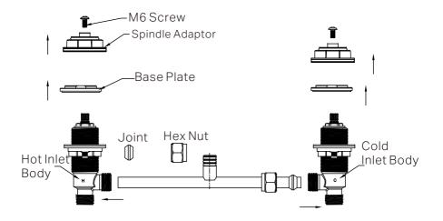
5. Carefully disassemble all components in the order illustrated above. Attach the Hex nuts and joints to the copper tee piece.
