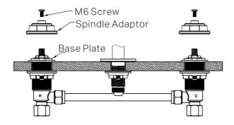
7. Screw the spindle adaptors onto the spindles and secure them with the M6 screws.
