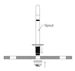
4. Insert the spout into the counter-top hole.
