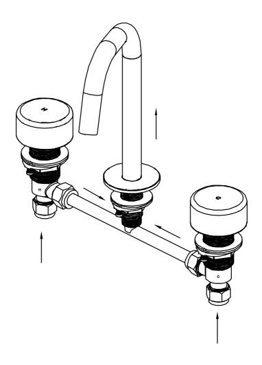
10. Turn on the drainage system and water supply, and inspect all connections for any signs of leakage.
