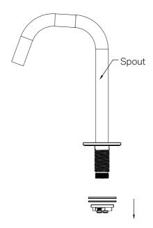
2. Remove the locking nut, metal washer, and rubber washer from the spout.
