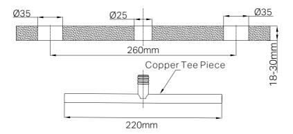
Note: The copper tee piece can be cut to a minimum length of 160mm to customize the distance between the hot and cold handles.
