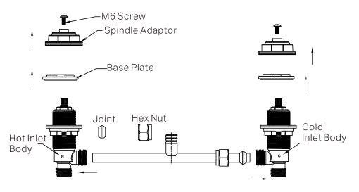
5. Carefully disassemble all components in the order illustrated above. Attach the Hex nuts and joints to the copper tee piece.
