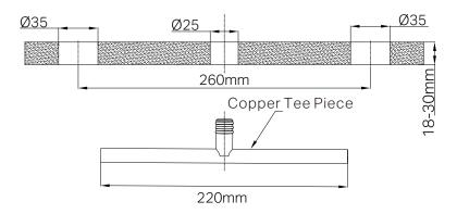
Note: The copper tee piece can be cut to a minimum length of 160mm to customize the distance between the hot and cold handles.
