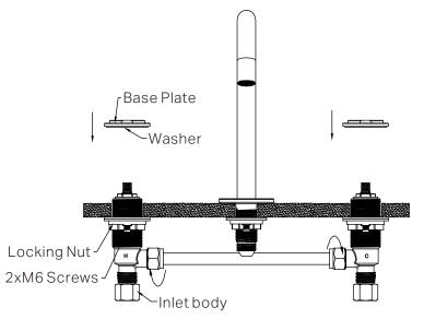
6. Insert the body set from underside of the counter-top. Using base plate and M6 screws to securing the body set, ensuring a firm connection. Ensure the washer is properly seated between the base plate and the body set.
