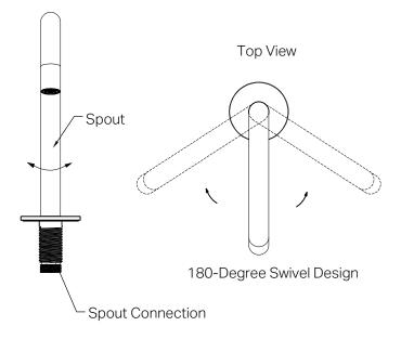
3. Secure the spout assembly at the spout connection.
