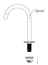
2. Remove the locking nut, metal washer, and rubber washer from the spout.
