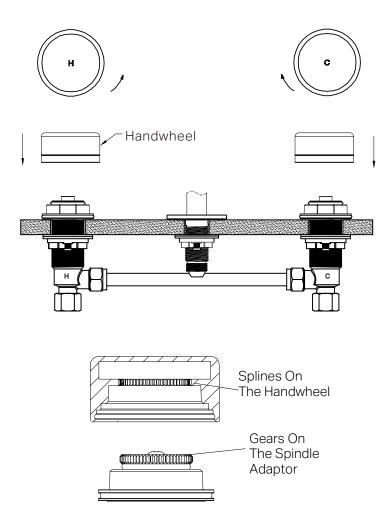
9. Align the Handwheels with the Spindle Adaptors:
