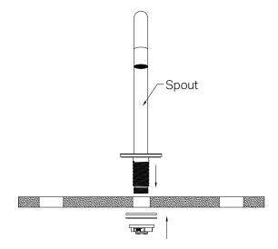
4. Insert the spout into the counter-top hole.
