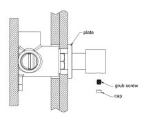
8.Put knob onto divertor ,tighten grub screw of knob firmly by hex wrench, put cap into knob.
