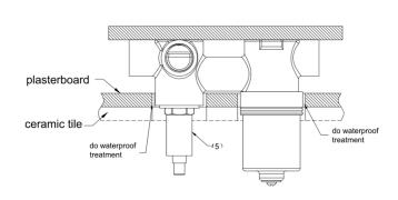
7.Install sleeve onto divertor, do waterproof treatment for gap of plasterboard and body.
