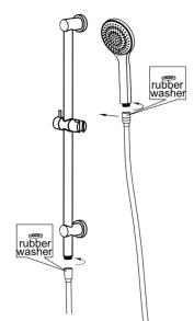
5. Connect shower rail and hand shower with hose. TEST & CHECK FOR LEAKS.
