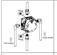
1.Connect the pipe to the water port, Left (H) for hot water and right (C) for cold water, top and bottom for mixed water.Plug the bottom or top mixed water outlet with the block if it's not required to use (single way valve).
