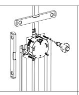
2-1.Get the wall cut accordingly to the instruction, check the horizontality and verticality of the valve box, adjust if necess-ary. Then Fix the valve box onto the wall.
