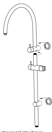
3. Screw shower rail into shower arm component. Tighten firmly. Push 2 back plates onto shower arm component and lower mounting pillar.
